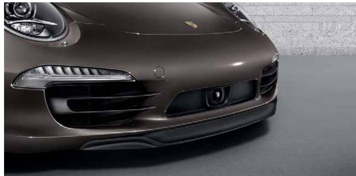
Radar sensor of Adaptive Cruise Control
