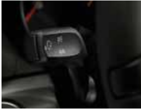
Voice-control system for PCM
