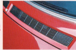
Flo-thru ventilation system (standard).
