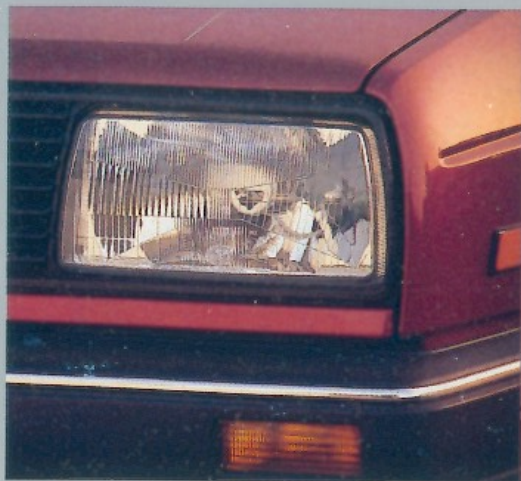
Eurostyle aerodynamic headlights help lower Jetta's drag coefficient to 0.36.
