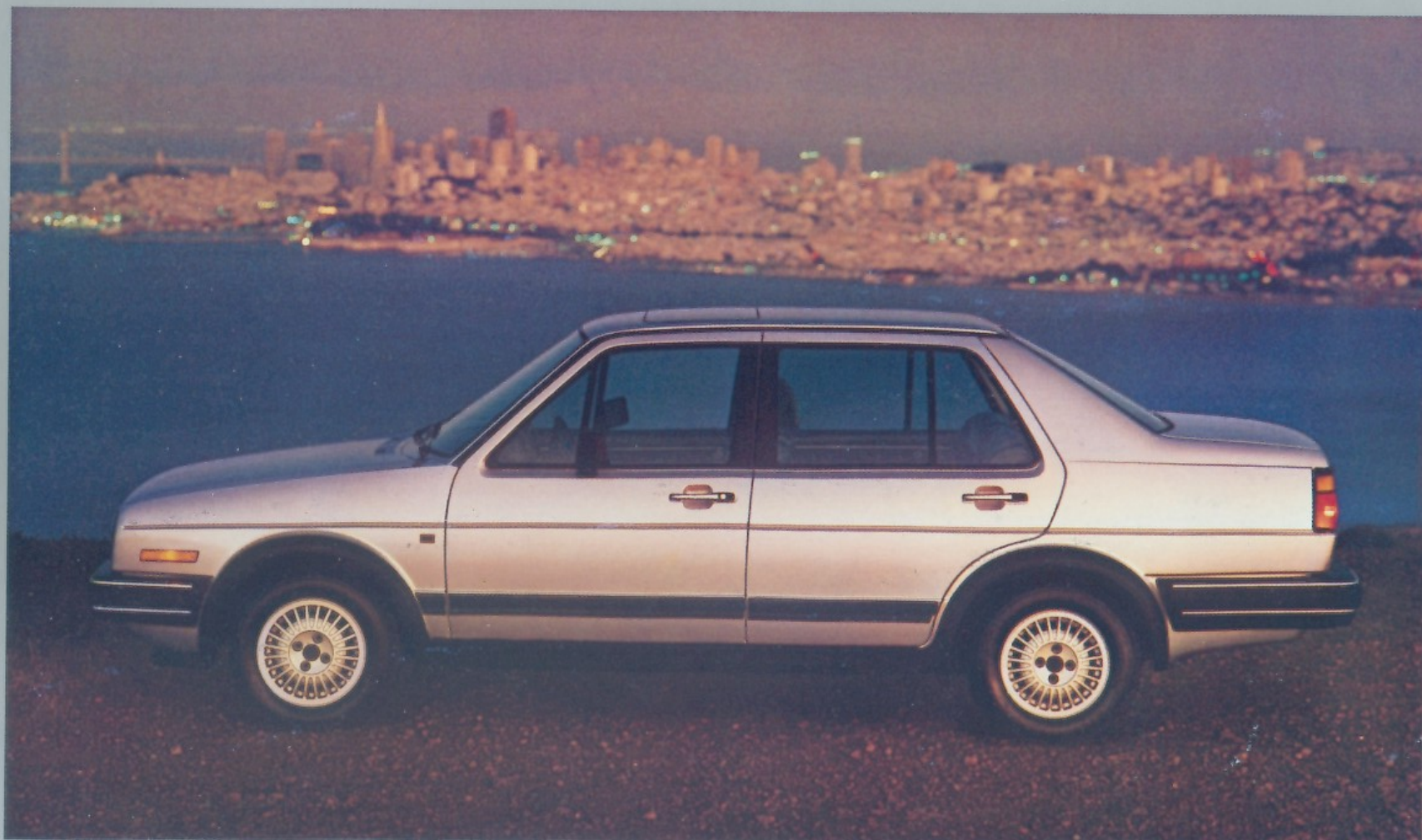
Eurostyle aerodynamic headlights help lower Jetta's drag coefficient to 0.36.
