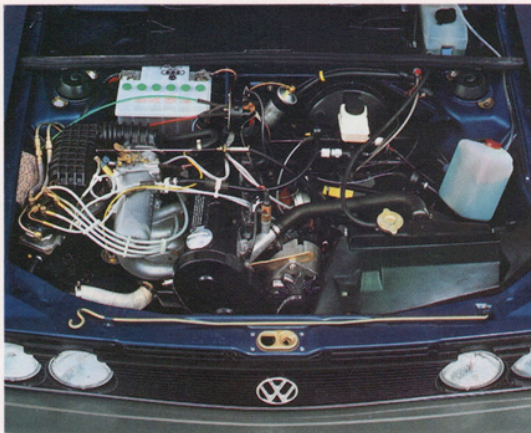
FUEL INJECTED, 1.6 LITER OVERHEAD CAM ENGINE.
