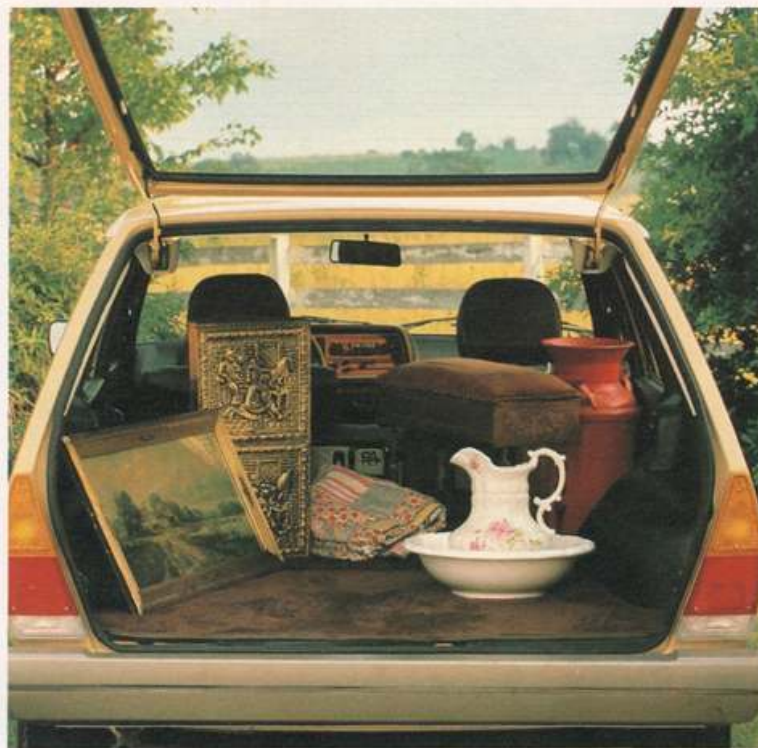
The tailgate goes all the way down to floor level, so there's no lip to hinder loading.
