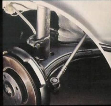
McPherson strut with long-travel coil/shock absorber.
