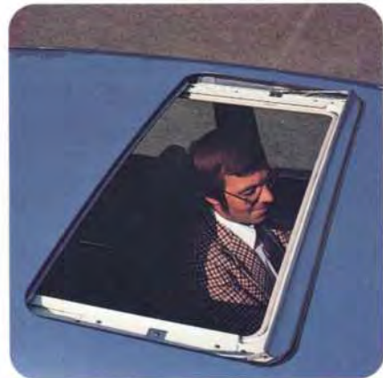
SLIDING STEEL SUNROOF WITH A BUILT-IN WIND DEFLECTOR IS STANDARD ON ALL GLE SEDANS.
