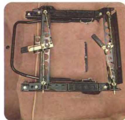
THE VOLVO FRONT SEAT FRAME IS SECURELY ANCHORED AT FOUR POINTS.
