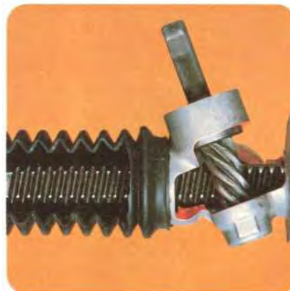
RACK AND PINION STEERING IS CONSIDERED BY MOST EXPERTS TO BE THE MOST PRECISE SYSTEM AVAILABLE.
