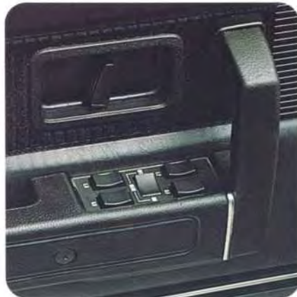
POWER WINDOWS ARE STANDARD ON GLE MODELS AND THE GL AND BERTONE COUPE. THE NEW CONTROLS ARE IN THE DRIVER'S ARMREST.
