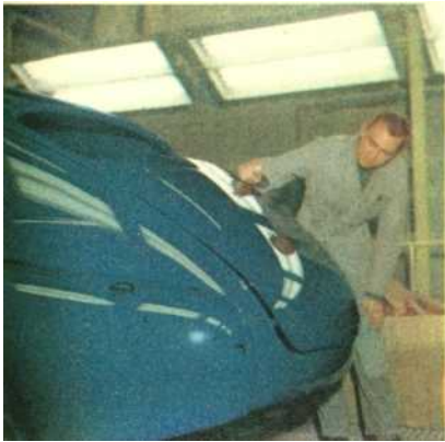
Inspection of enamel top coat.
