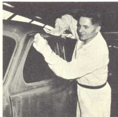
Inspection of enamel base coat after sanding.
