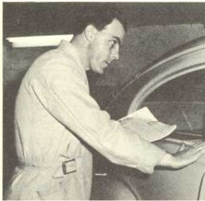
Final inspection of all painted surfaces.
