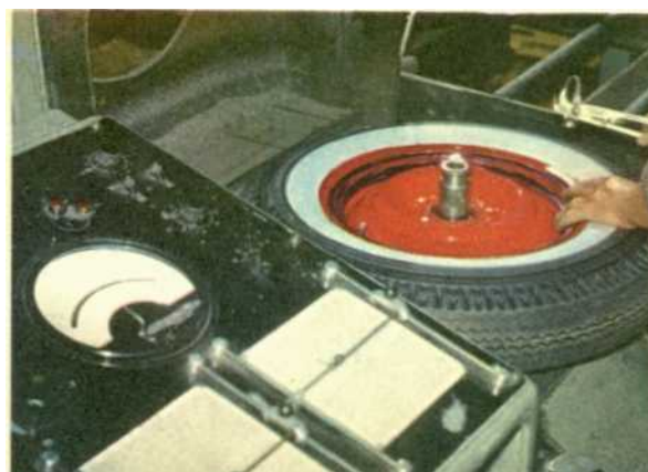
All wheels are balanced at the Volvo plant before assembly-a guarantee of maximum safety and minimum tire wear.
