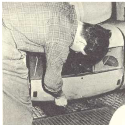
Inspection of enamel base coat after spraying.
