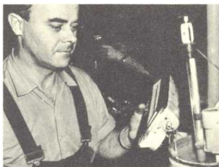
Inspection of coolant thermometer for correct reading.
