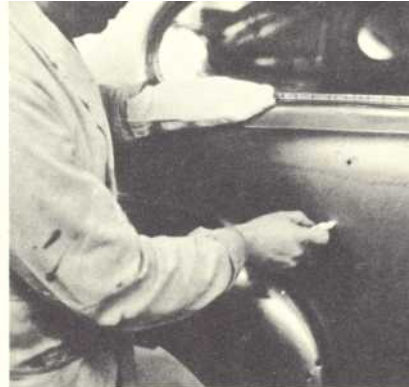
Inspecting metal on newly-arrived bodies after degreasing.
