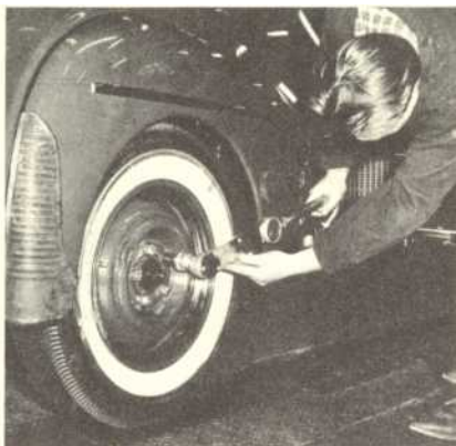
Final inspection of all functions: checking wheel nuts with torque-wrench.
