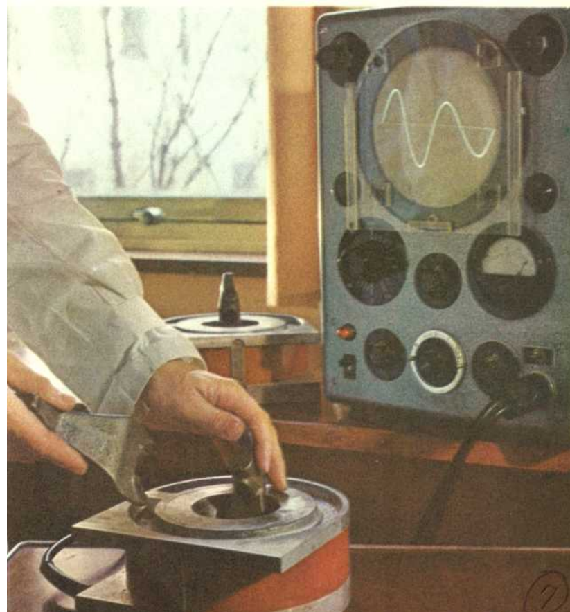
Testing Volvo gearshift forks electroinductively in a Magnaflux machine.
