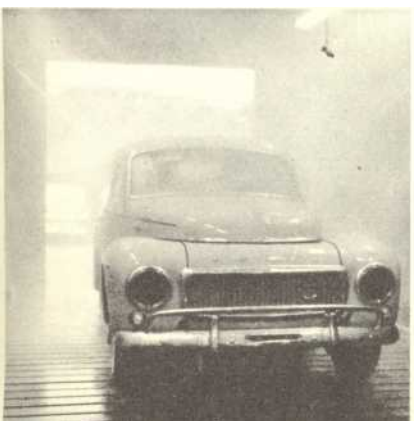
The water test. If the car gets through this high-pressure water dunking, it's not likely to leak later.
