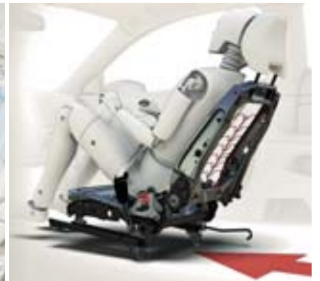
Whiplash Protection System (WHIPS)
