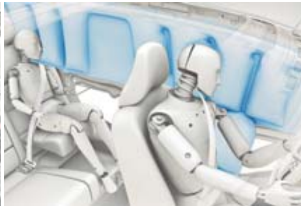
Inflatable Curtain (IC)
