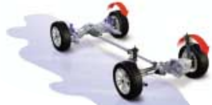
If one or both wheels on one side of the vehicle spin, more power goes instantly to the wheels with better traction.
