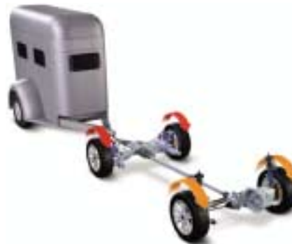
If you carry heavy loads, the rear wheels receive more power to maximize driving stability.
