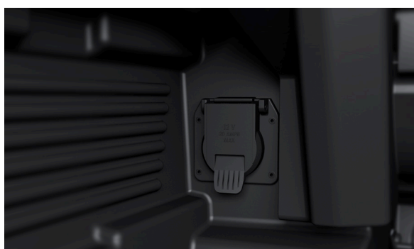
Bedliner with 12V power socket
