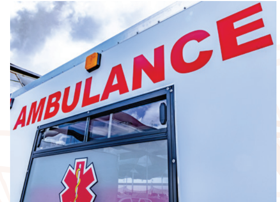
AMBULANCE DECALS AND SLIDING WINDOWS WITH 4MM TOUGHENED FROSTED ARMOUR PLATE GLASS
