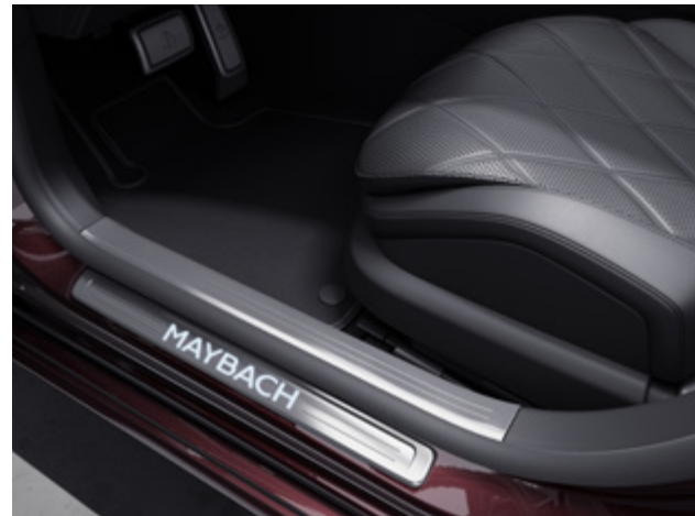
Door sill panels with "Maybach" lettering at front and rear, illuminated (U25)
