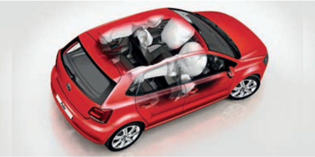
The advanced airbag system features two side airbags and driver and front passenger airbags with front passenger airbag deactivation.
