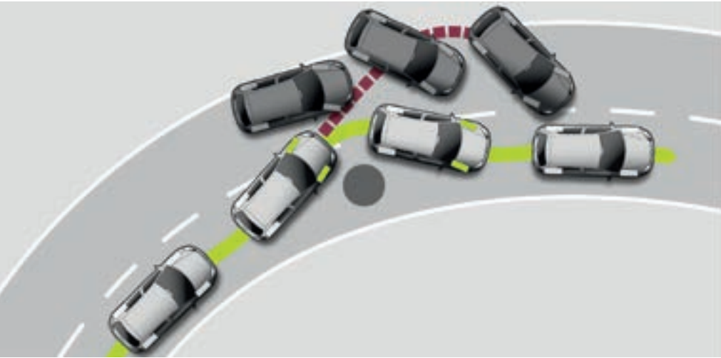
Electronic Stability Programme (ESP) intelligently controls the engine management system to help correct oversteer, understeer and loss of grip when turning.
