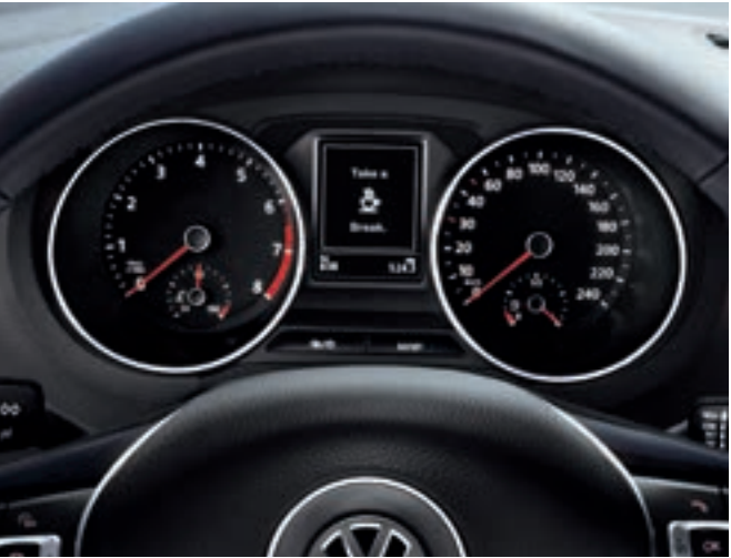
Fatigue Detection (standard on Highline) detects irregular driving patterns, and warns you when it's time to take a break on a long drive.
