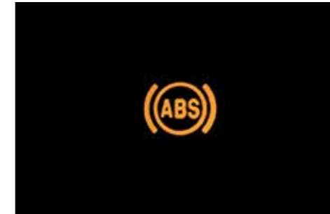
By helping prevent wheel lock when you apply the brakes suddenly, the ABS helps enhance handling and driving safety
