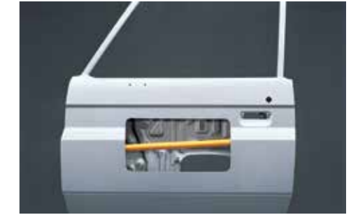
Side impact beams reduce the likelihood of side impact intruding through the doors
