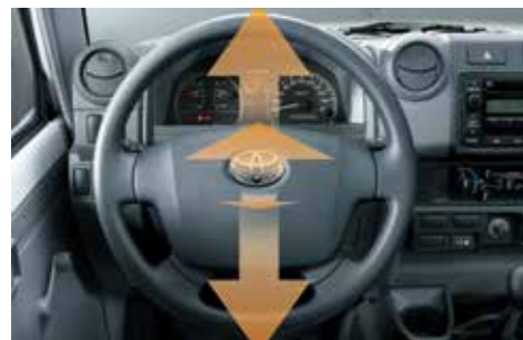
A tilt-adjustable, telescoping steering wheel allows finer adjustments to maximise driving comfort
