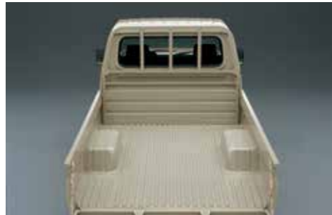
Guard frames protect the cabin from shifting cargo
